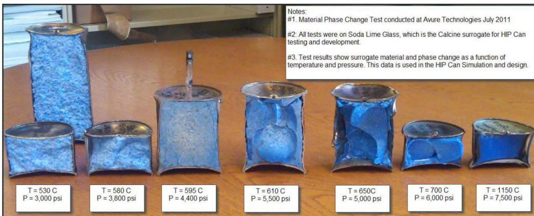
Fig. 17. Volume reduction cases at various conditions.
