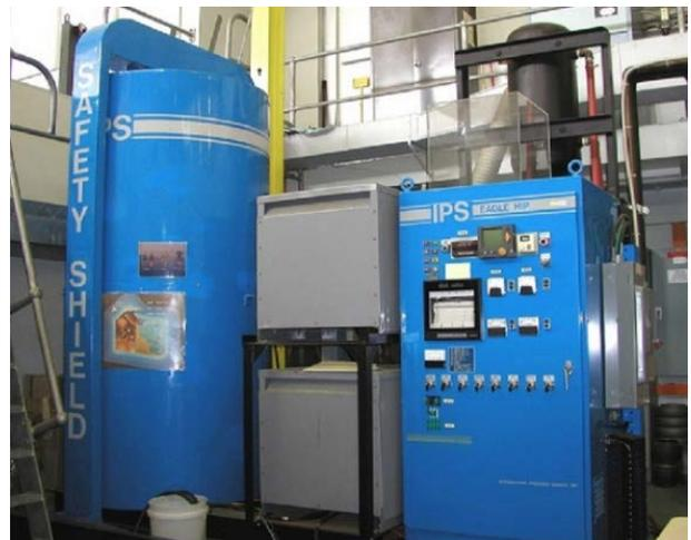
**Fig. 18.** ANSTO HIP equipment (Pressure: 200 MPa).
